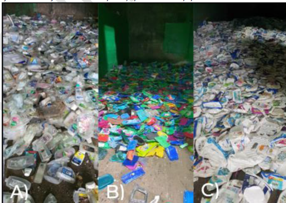
Figure 11: Non-food material after a hand sort. A) Clear, B) Multi-coloured, C) White.
