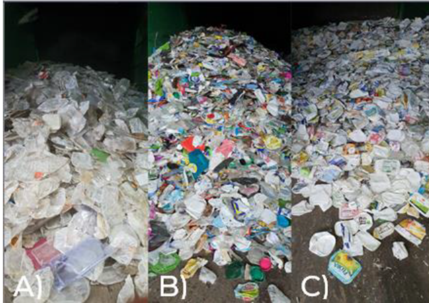
Figure 10: Food grade material after a hand sort. A) Clear, B) Multi-coloured, C) White
