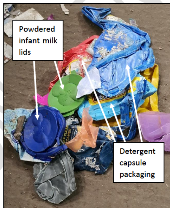
Figure 12: Multi-coloured PP classified as non-food use PP during multi-coloured PP feedstock audits
